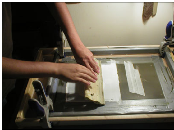
Fig. 11.4 Manual screen printing process
